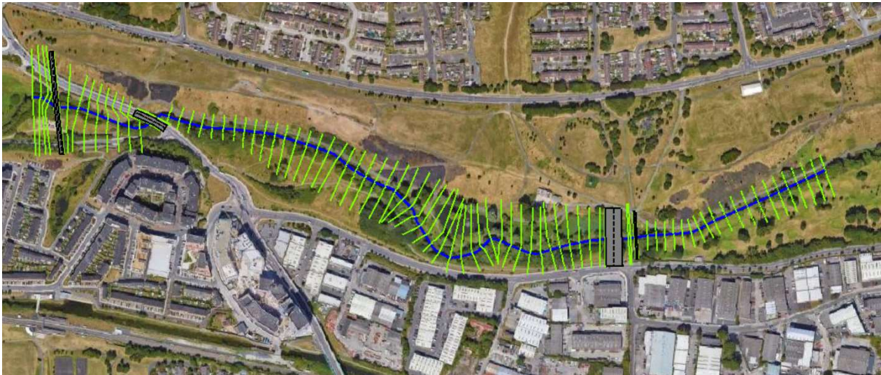
Figure 5.6: Stretch of river extents modelled and location of the river stations.
